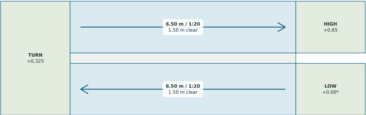
RA: 10.50 x 3.30 m clear layout; allow about 10.80 x 3.60 m overall
